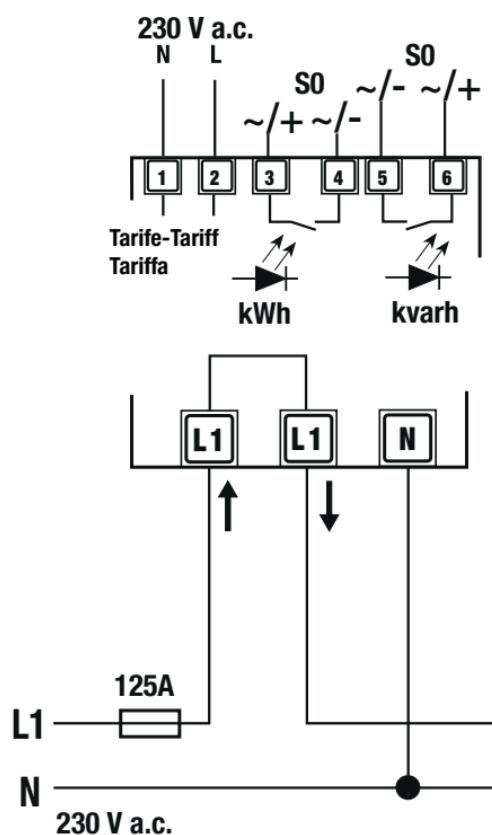
A fuse of 125 A is recommended for the line protection.
